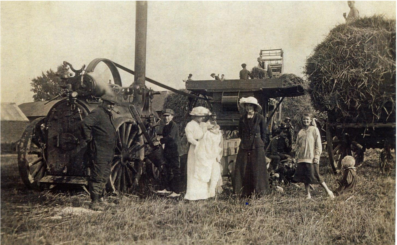
c1915: Brickhouse Farm, West Mersea. William Trim (left) was a threshing contractor at Mersea. The steam engine was a 'portable', i.e. it was not self-propelled and had to be pulled by a horse. The young man with cap is Horace Whiting. Teenage girl is Catherine Vince (Mrs George), born 8 Nov 1899.
